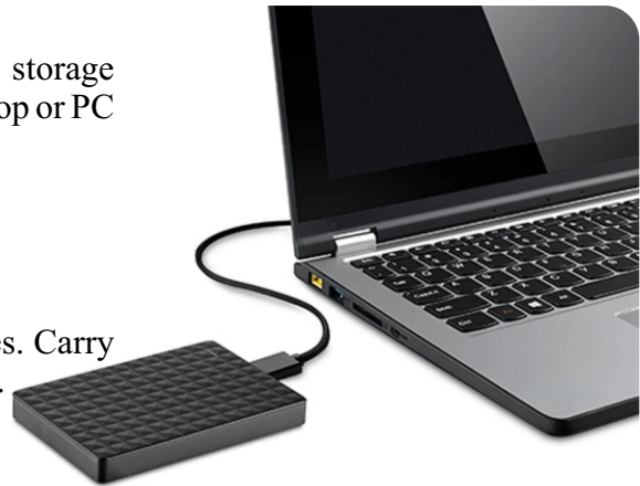
Figure 1.21 shows an External drive connected to the Laptop through the USB port
