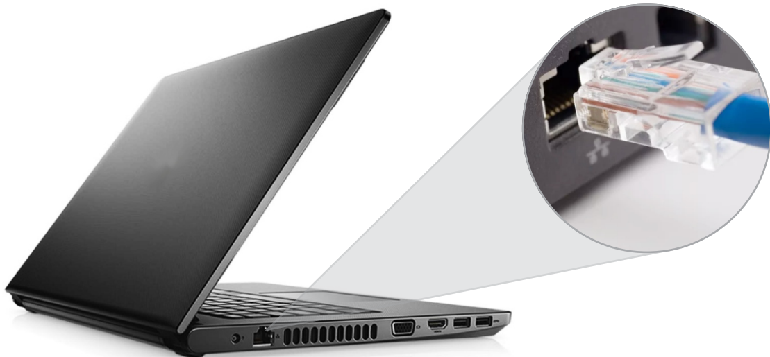
Figure 1.2 Ethernet Port and cable
