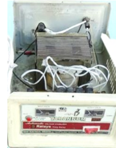
Fig: 16.20 Transformer in stabilizer
