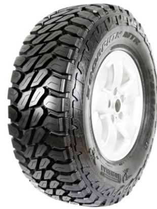
Fig. (3.18) (a) Tyre Grooves improve grip on road
